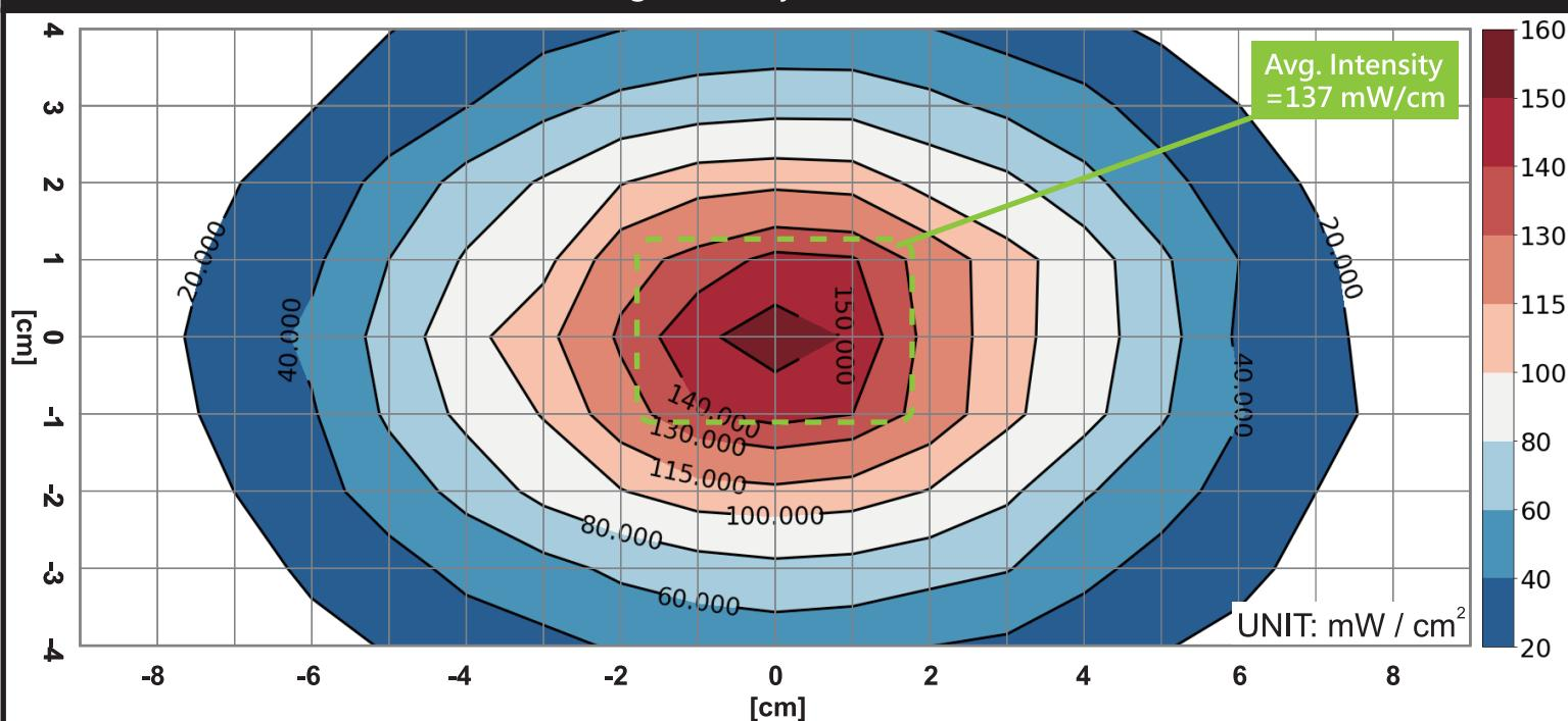
\* Intensity values are the average of PR160/PR160L-390nm, PR160/PR160L-427nm, PR160/PR160L-440nm, PR160/PR160L-456nm, and PR160/PR160L-467nm. Such values do not apply to PR160/PR160L-370nm
