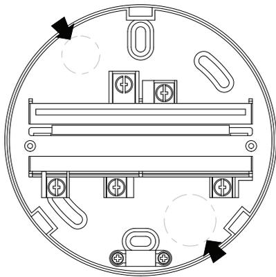
Drilled hole allows the wire to pass through.
